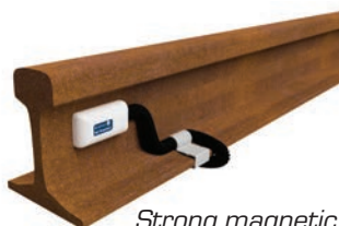
Strong magnetic temperature sensor:
