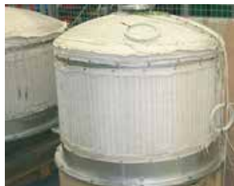
Vessel for polyol and isocyanat for the production of PUR foam.
