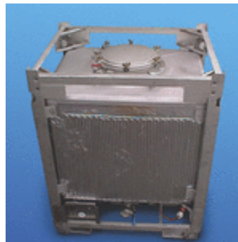
1000 l transport container before mounting of insulation
